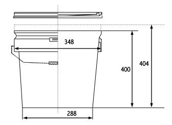
Measurements in millimetres
